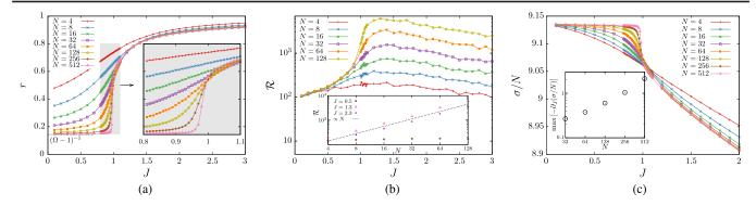
FIG. 2. Observables for the mean-field variant as functions of the interaction strength *J*. (a) Order parameter *r* indicates the onset of subharmonic synchronization above the critical point. (b) Number of coherent oscillations  $\mathcal{R}$  diverge in thermodynamic limit below the critical point. (c) Rate of entropy production per unit  $\sigma/N$ ; its first derivative diverges at criticality in the thermodynamic limit, as shown in the inset.
